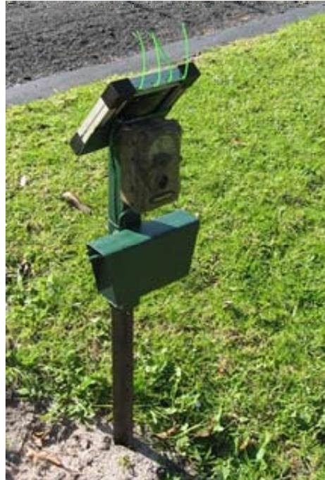
A final consideration is the weight of the whole unit. Because we are installing the units off-track, we will be carrying these into the bush and a neat, lightweight unit will be needed.
