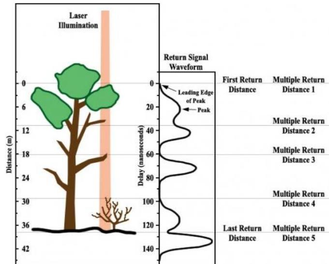
Figure 7. Full waveform system.
